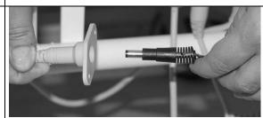
WITH THE ONE HAND, YOU GRAB AROUND THE CHARGING PLUG (SOCKET) ON THE CHAIR AND WITH THE OTHER HAND, YOU PUSH THE PLUG FROM THE TRANSFORMER IN PLACE.
