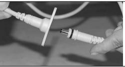
WITH THE ONE HAND, YOU GRAB AROUND THE CHARGING PLUG (SOCKET) ON THE CHAIR AND WITH THE OTHER HAND YOU PULL OUT THE CONNECTING CABLE FOR THE BATTERY.
