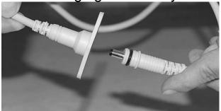
With the one hand, you grab around the charging plug (Socket) on the chair and with the other hand you pull out the connecting cable for the battery.
