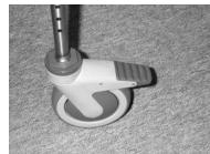
The right front wheel can be locked the direction. Use of this makes it easier to start and moving the chair.
