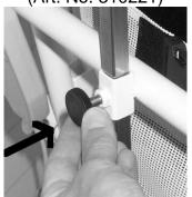
The height of the headrest is adjusted by loosening the finger screw and tightening it again when the height is right.
