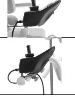
The joystick can be placed at the front so the user can control it or at the back so the helper can control is. You fasten it to the chair by tightening the finger screw.
